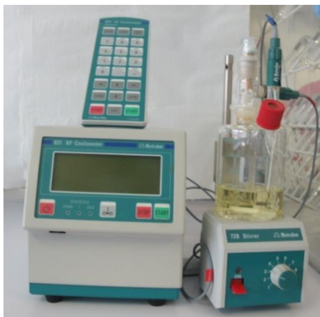
Figure 10 Metrohm 831 Karl Fischer Coulometer.
